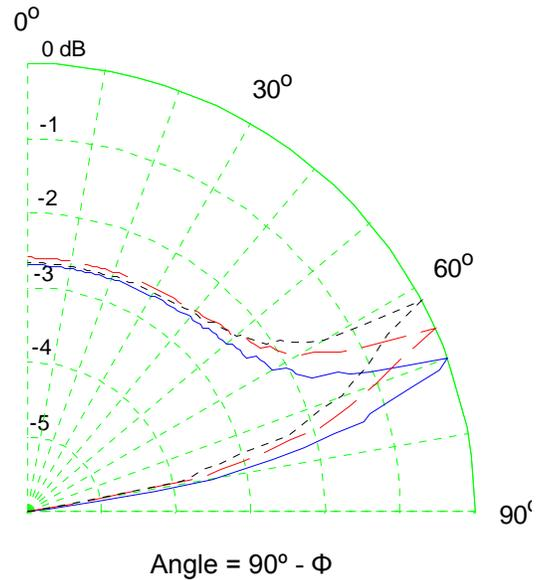
Fig. 5. Directionality of snap energy measured at  $c_1 = 1600$  (solid), 1650 (dashed), 1700 (dotted) m/s with  $\delta = 2$  cm,  $\rho_1 = 1800$  kg/m<sup>3</sup>
