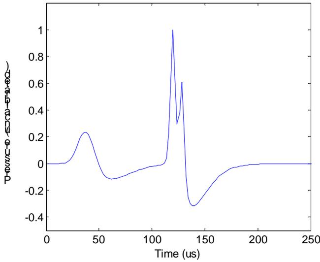
Fig. 3. Simulated snap with at  $\Phi = 21^\circ$ ,  $\delta = 1.5$  cm,  $c_1 = 1600$  m/s,  $\rho_1 = 1800$  kg/m<sup>3</sup>
