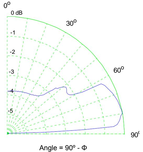
Fig. 6. Directionality of snap energy measured at  $\delta = 10$  cm,  $c_1 = 1700$  m/s,  $\rho_1 = 1800$  kg/m<sup>3</sup>
