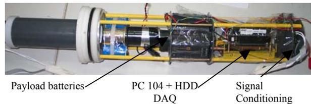
Fig. 10. Modified APV payload with the data acquisition system
