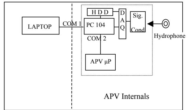
Fig. 9 Block diagram showing interconnections between different electronics blocks
