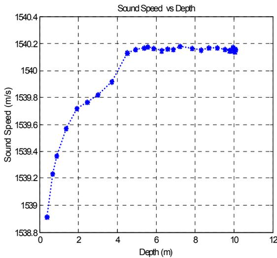
Fig.11 Sound speed vs. depth
