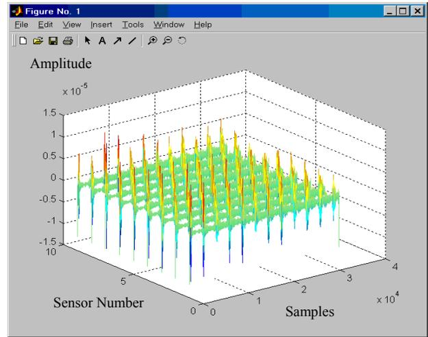
Figure 6. The receivers at the other end receive a multi path reflection of all the pulse trains sent by the source.
