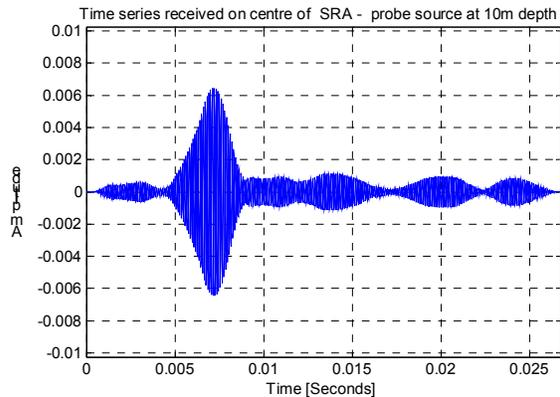
Fig.0 Single Pulse received at Rec. Source Array
