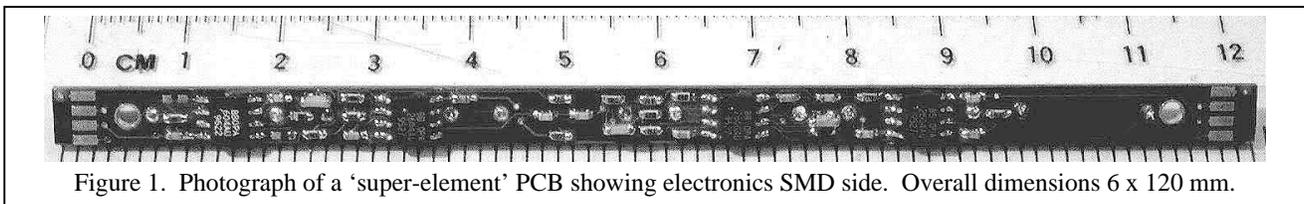
pass the PCB, keeping the cross section to a minimum and reducing diffraction problems. Super-elements are linked by copper wires and a wire or monofilament nylon strain relief. Longer prototypes would probably require carbon fibre or kevlar stranded strain relief. A picture of an assembled super-element PCB is shown in Fig. 1.
