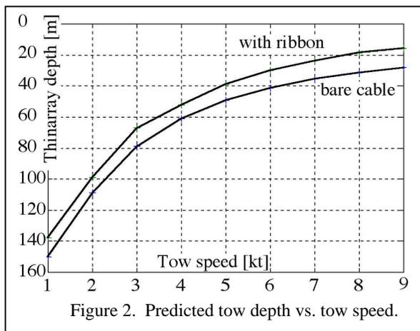
Figure 2. Predicted tow depth vs. tow speed.
