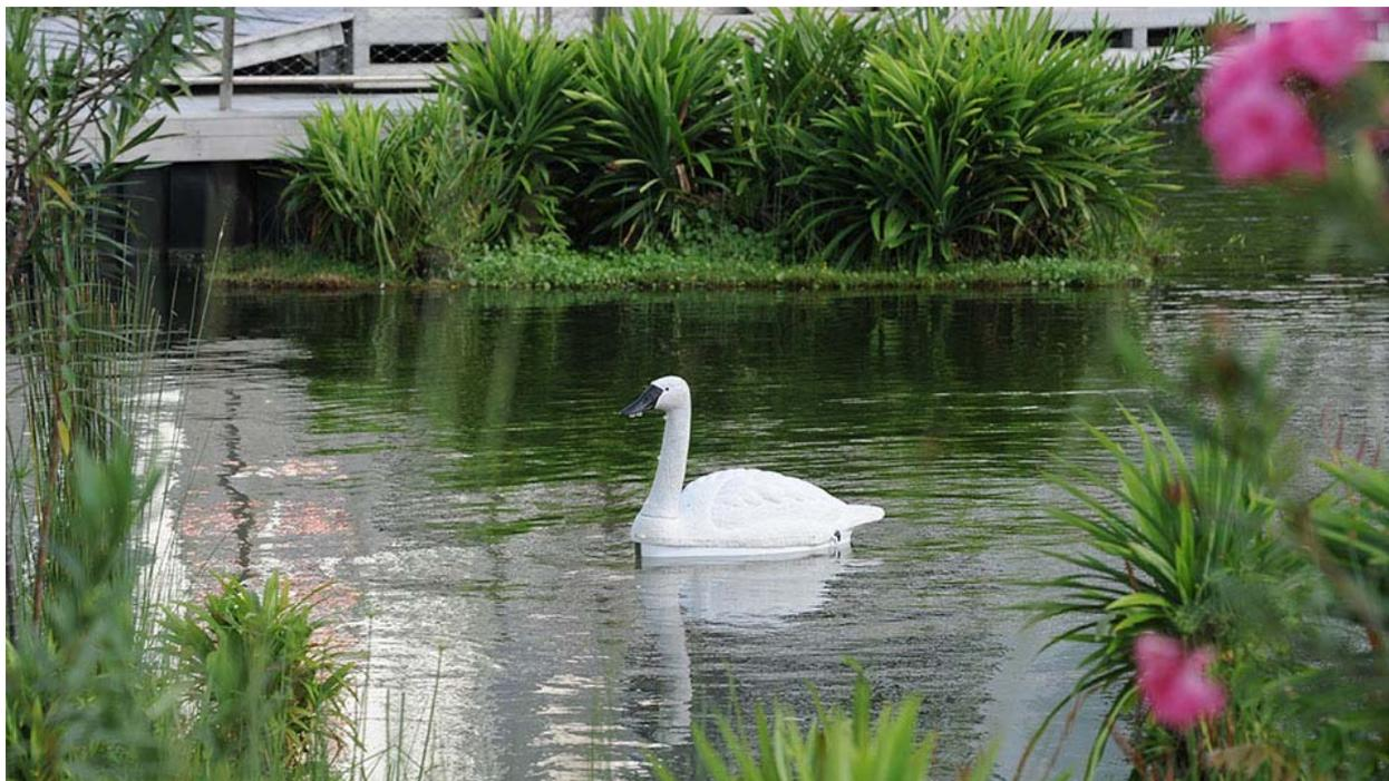
This robotic swan collects real-time water-sampling data cost-efficiently
