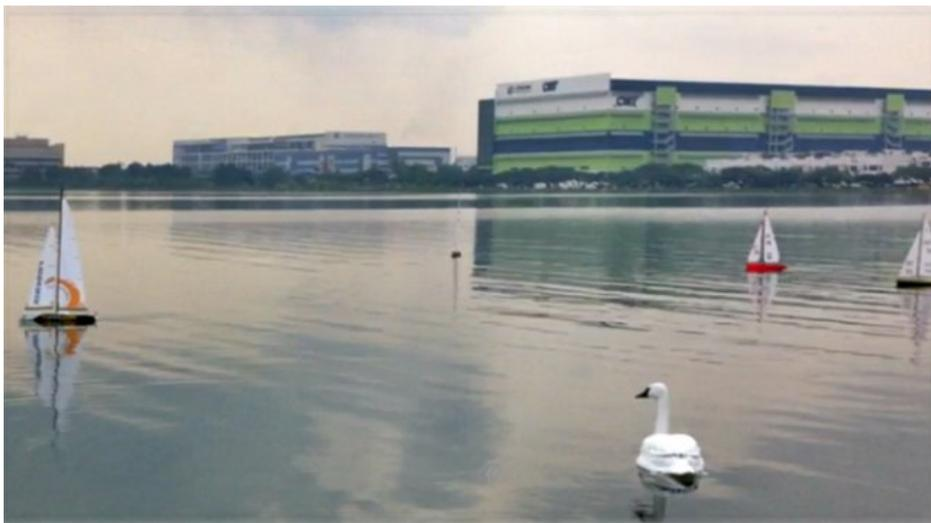
Each bird-bot has a GPS receiver for navigation. That allows the bots to methodically move around a body of water and make sure different areas get tested without unnecessarily duplicating data points, while also letting them return on their own to a charging station — all of which minimizes the time researchers need to spend on direct remote control and maintenance. Data can be collected by Wi-Fi
