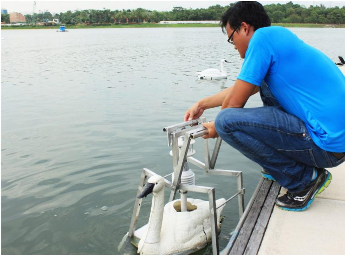
As the swans float on the water, wireless technology is used to stream real-time data results to a command centre. The actions of the swans can then be remotely altered by operators based on this data.
