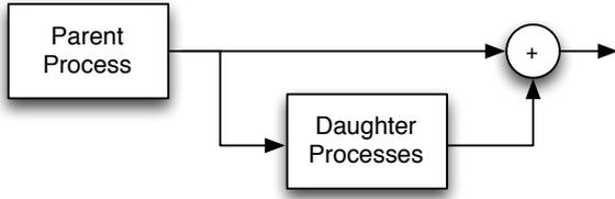
Fig. 11. Block diagram of the overall error generation process model.
