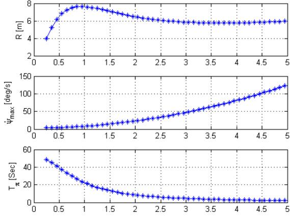
Fig. 13. Turning radius of AUV at different speeds
