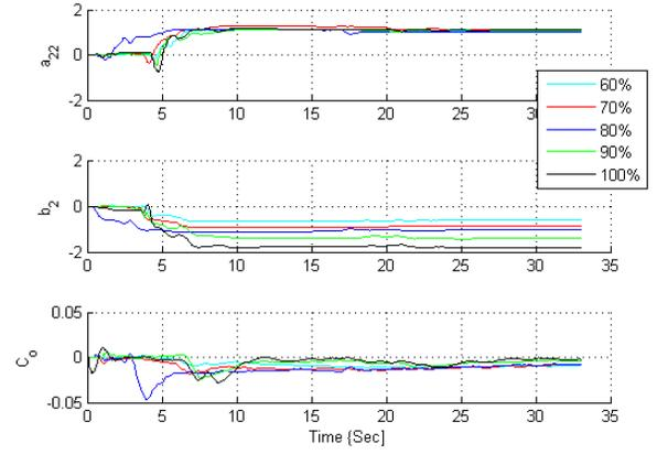
Fig. 9. Online parameters estimation of yaw dynamics for different thrusts
