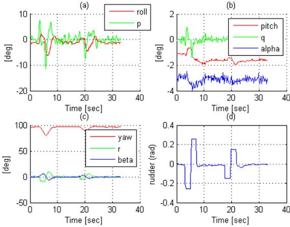
Fig. 8. Experiment run for identification for yaw dynamics at 70% thrust. Plot of roll, pitch, yaw and rudder
