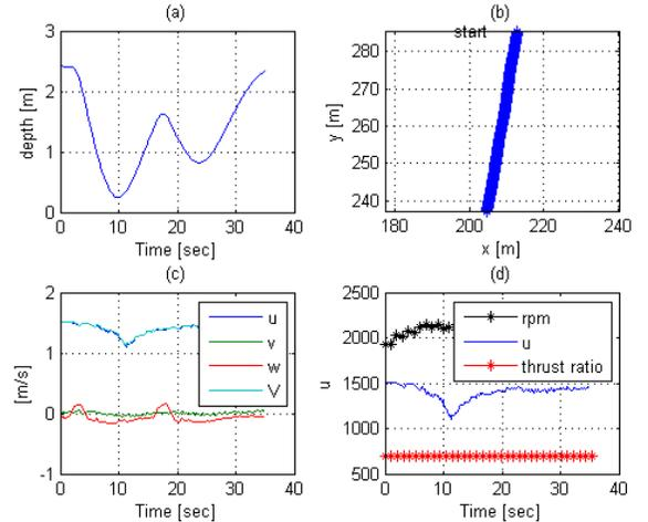
Fig. 3. Experiment run for identification for pitch dynamics at thrust ratio 70%. Plot of depth, x-y position, velocity and thrust ratio
