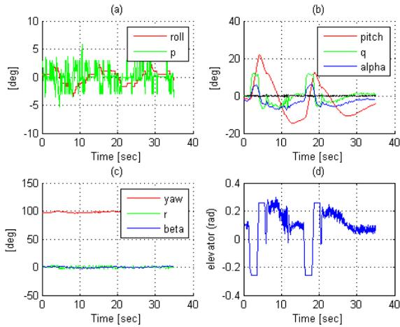
Fig. 4. Experiment run for identification for pitch dynamics at thrust ratio 70%. Plot of roll, pitch, yaw and elevator
