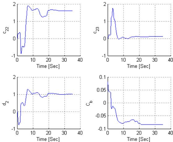
Fig. 5. Online parameters estimation of pitch dynamics at 70% thrust
