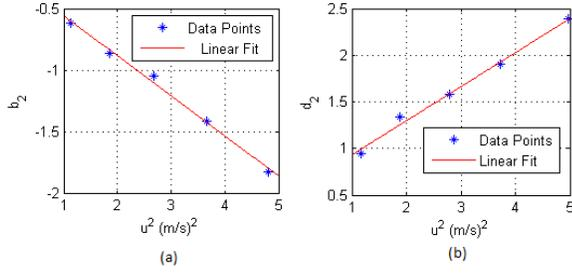
Fig. 10. (a) Plot of rudder control authority  $b_2$  against speed<sup>2</sup> (b)Plot of elevator control authority  $d_2$  against speed<sup>2</sup>
