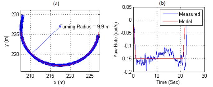
Fig. 14. (a) Turning radius of AUV during the case study (b) Measured yaw rate and modeled yaw rate during the U-turn
