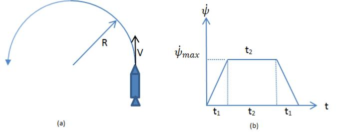
Fig. 12. (a) Turning Radius  $R$  of an AUV travel at speed,  $V$  and (b) Trapezoidal Profile for Yaw Angular velocity
