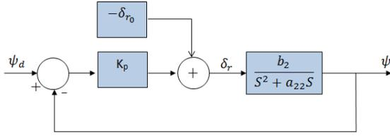
Fig. 15. Block Diagram for Heading Control
