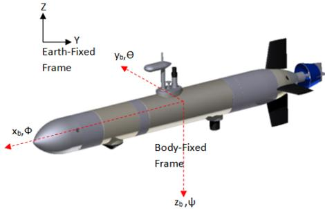
Fig. 1. Reference frame of STARFISH AUV.
