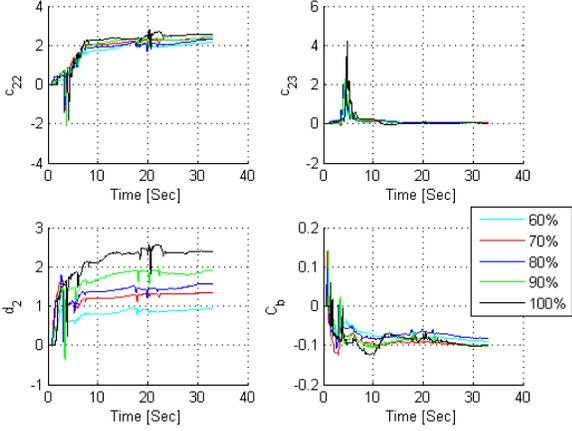
Fig. 11. Online parameters estimation of pitch dynamics for different thrusts
