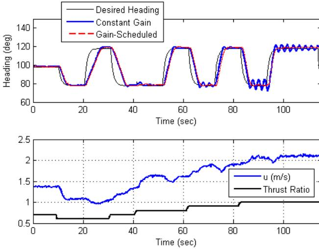
Fig. 16. Experiment results for heading control under constant gain controller and gain-scheduled controller
