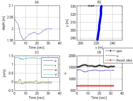
Fig. 7. Experiment run for identification for yaw dynamics at 70% thrust. Plot of depth, x-y position, velocity and thrust ratio
