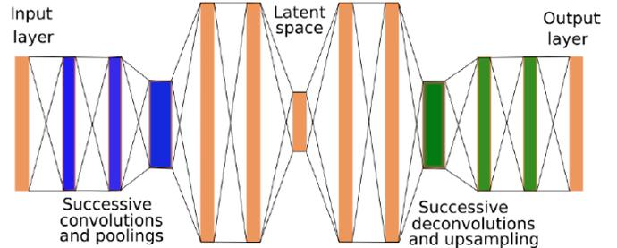
Fig. 2. Structure of the convolutional AE used. Blue blocks denote the convolutional layers in the encoder, green ones denote those used in the decoder, and orange blocks denote fully connected layers.
