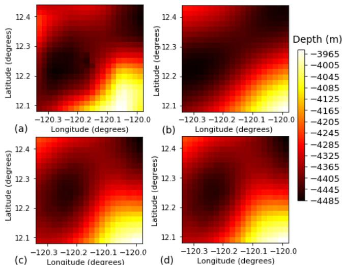
Fig. 3. Bathymetric maps around the location 12.25°N, 120.15°W: (a) original bathymetric map; encoded and reconstructed maps using (b) PCA, (c) AE trained based on mean-square error, and (d) AE trained based on maximum-absolute error.
