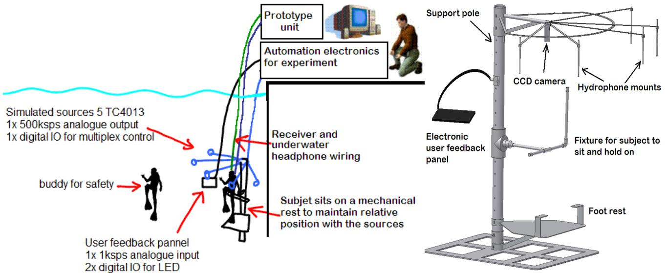
Figure 5: Experiment setup of swimming pool experiment
