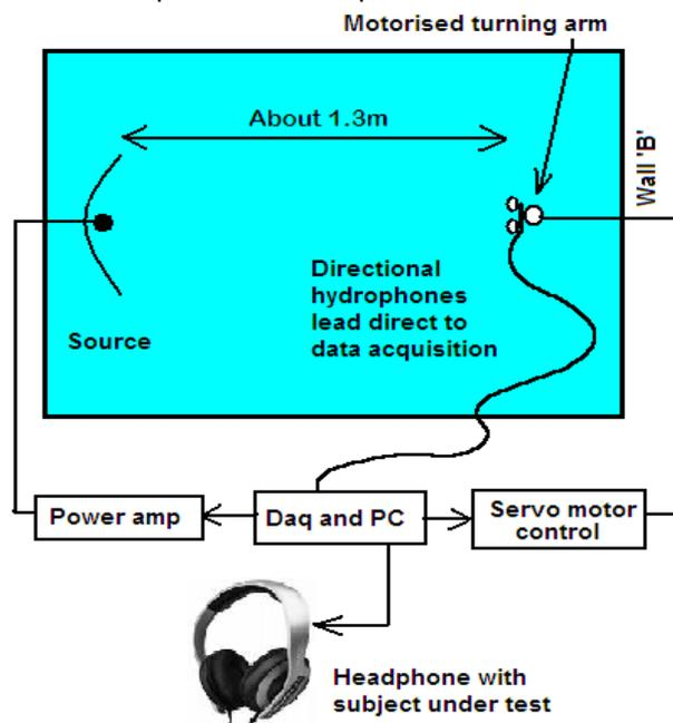
Figure 1: Schematics of the tank experiment
