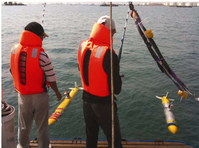
Fig. 4—Two heterogeneous STARFISH AUVs configured from the same basic vehicles. BlueStar with DVL payload (right) and RedStar with sidescan sonar payload (left). Fishing lines were attached to the AUVs in the initial trials to safe guard them.
