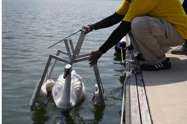
Fig. 1. Autonomous Surface Vehicle being deployed for monitoring and water sample collection in a freshwater lake in Singapore.
