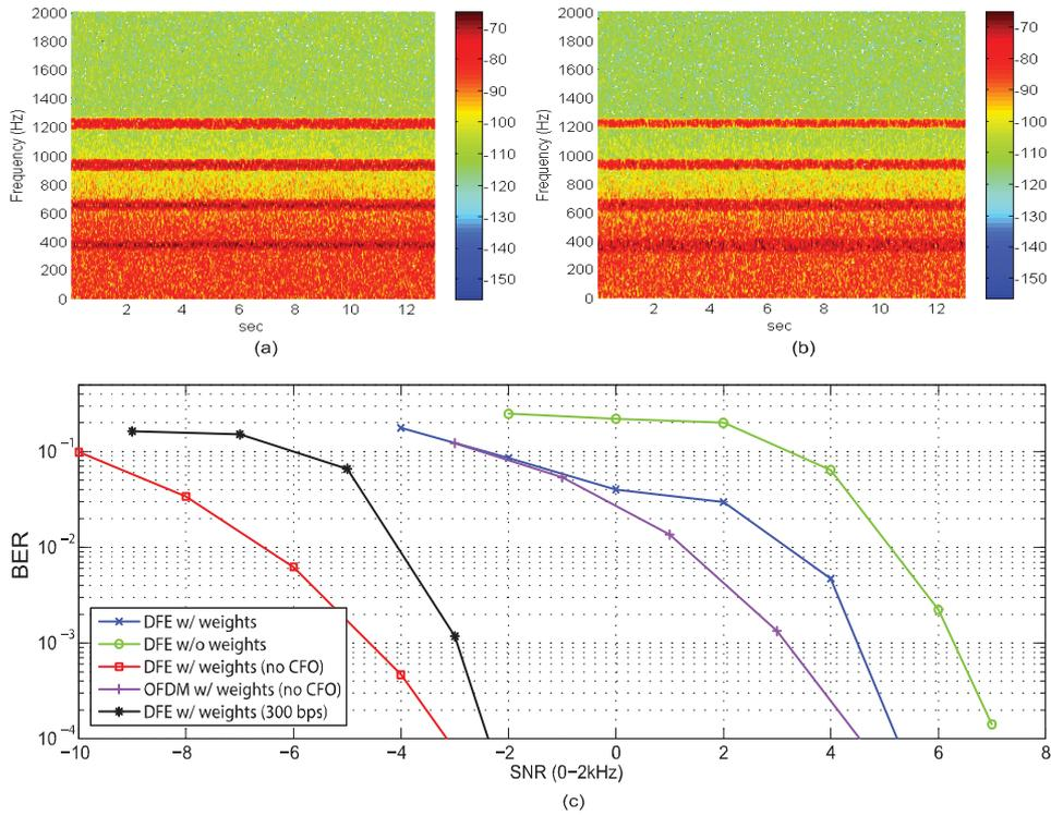
Fig. 3. (a) Spectrogram of the received multicarrier signal for 4 dB SNR. (b) Spectrogram of the received OFDM signal for 4 dB SNR. For both (a) and (b) the colorbar is in dB scale. (c) BER vs. SNR curves.
