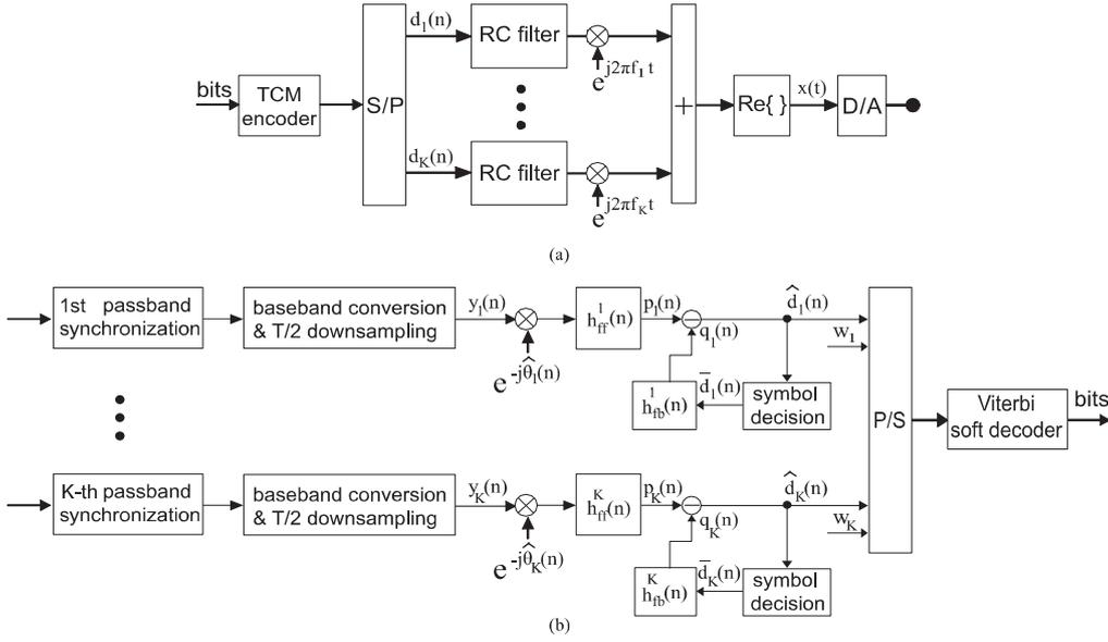
Fig. 2. Block diagram of the communications system: (a) transmitter; (b) receiver.
