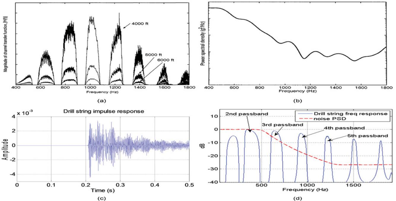
Fig. 1. (a) Drill string frequency response for various lengths (figure is taken from [6]). (b) Experimental noise PSD (figure is taken from [6]). (c) Simulated channel impulse response of 1 km steel drill string. (d) Simulated channel frequency response and noise PSD. Both plots are normalised to 0 dB.
