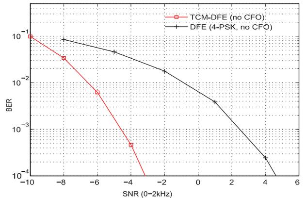
Fig. 4. Comparison of the proposed TCM-DFE system with uncoded 4-PSK DFE system.
