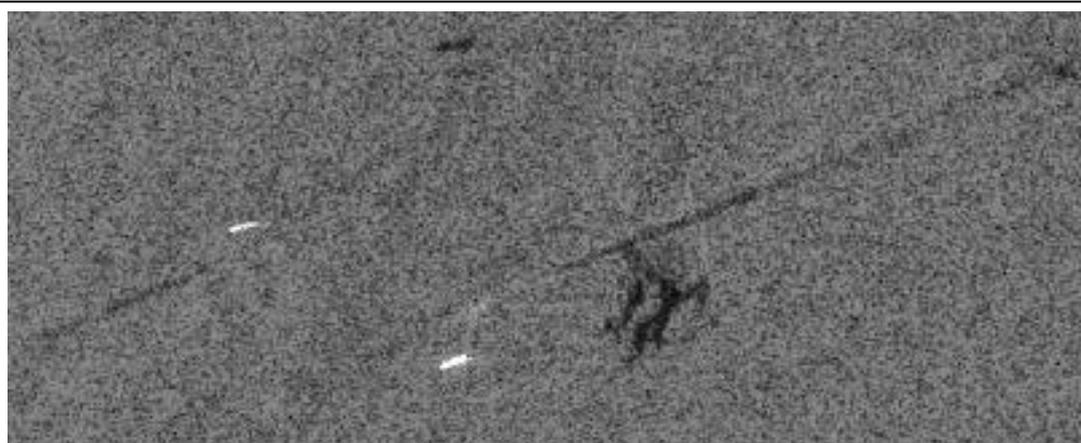
Figure 1. ERS-2 SAR image (original copyright ESA 1996) showing two ships and their turbulent wakes. The wakes are offset from the ships' headings due to SAR processing artefacts, from which ship speed can be inferred.
