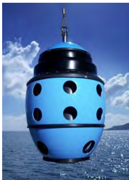
QinetiQ's Cerberus diver detection sonar.
