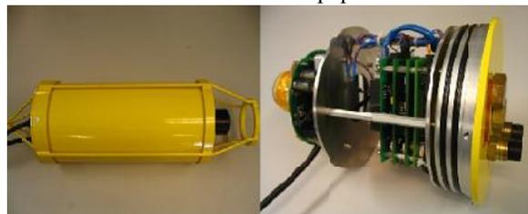
Fig. 2. The ARL modem used in the tests
