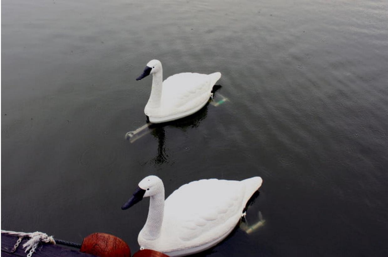
Water measurements which can be taken by the swans include water pH level, dissolved oxygen, turbidity, and chlorophyll. Due to the cloud connection, which analyzes the water data in real time, authorities can be alerted immediately if there is some reason why the local H<sub>2</sub>O may not be safe to drink. This is particularly useful in areas where dry weather prompts greater growth of algae, thereby making it more important to closely monitor water quality.
