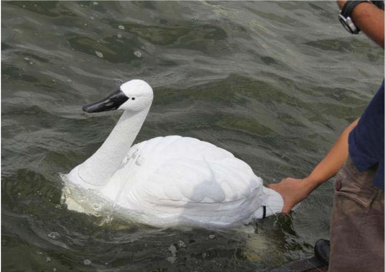
The NUSwans are tough enough not to break if they get a whack from a wayward oar or suffer a kayak collision, and upgrades are already planned. The addition of phosphate sensors, which the university has prototyped itself due to a lack of commercial availability, will let the NUSwan check for [algal blooms](#), which can choke water ecosystems.
