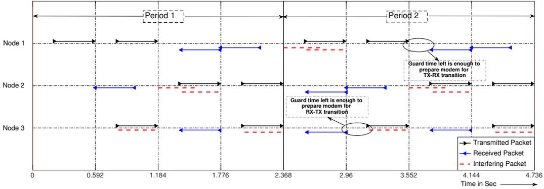
**Figure 4:** Schedule visualization with modem constraints (the guard times set in the time slot not only take care of the constraints due to geometry but also consider TX-RX and RX-TX transition times in modem).
