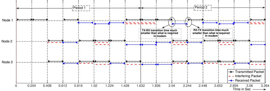
**Figure 3:** Schedule visualization without modem constraints (the guard times set in the time slot take care of only the early receptions and delayed receptions problem due to the approximations made in the delay matrix because of the network geometry).
