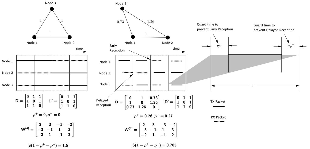
**Figure 1:** Effects of Approximation (Note that two different geometries adopt the same schedule but the guard times are essential to prevent packets being received across time slots. This illustrates the effect of approximating the non-integer delay matrix. The guard times at the start and end of the time slot can be expressed in terms of  $\rho^+$  &  $\rho^-$ .)
