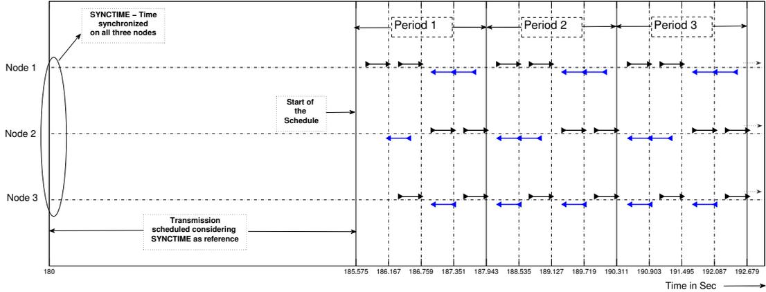
**Figure 7:** Schedule verified on UnetSim with modem model `ARLUNETModem` for time synchronization, accuracy of timed transmissions and reception times (the transmission and reception times used in the plot are taken from the clock notifications in the simulator [4].)
