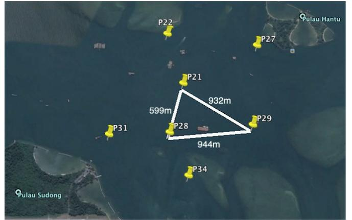
**Figure 2:** UNET network node locations during the MISSION 2013 experiment (deployment #1). Yellow markers are network nodes. The geometry considered for the case study is marked with the distances between the links.
