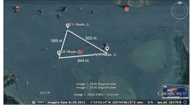
Fig. 2. UNET network node locations during the MISSION 2013 experiment (deployment #1). White markers are network nodes. The geometry considered for the case study is marked with the distances between the links.
