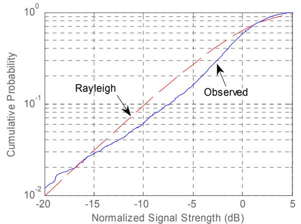
Fig. 7. Cumulative distribution function of signal strength showing fading behaviour of direct arrival at 50 m
