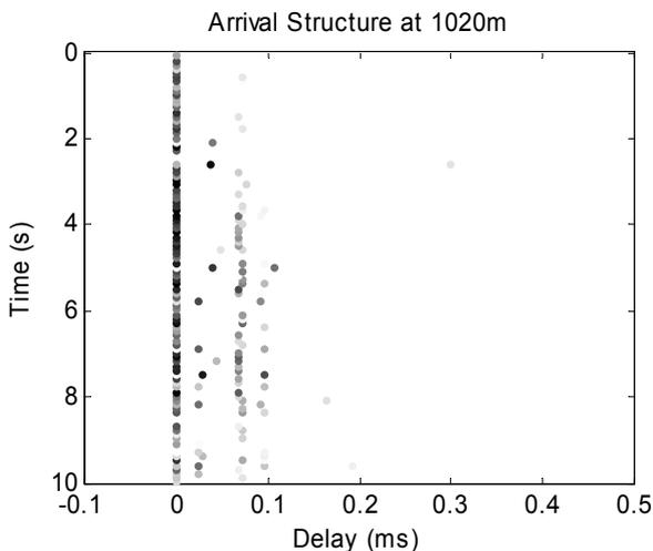
Fig. 8. Multipath arrival structure at 1020 m
