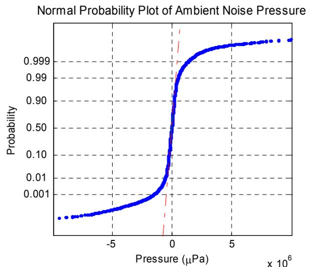
Fig. 1. A Normal Probability Plot of acoustic pressure of ambient noise recorded in Singapore waters shows severe deviation (heavy tails) from Gaussian distribution
