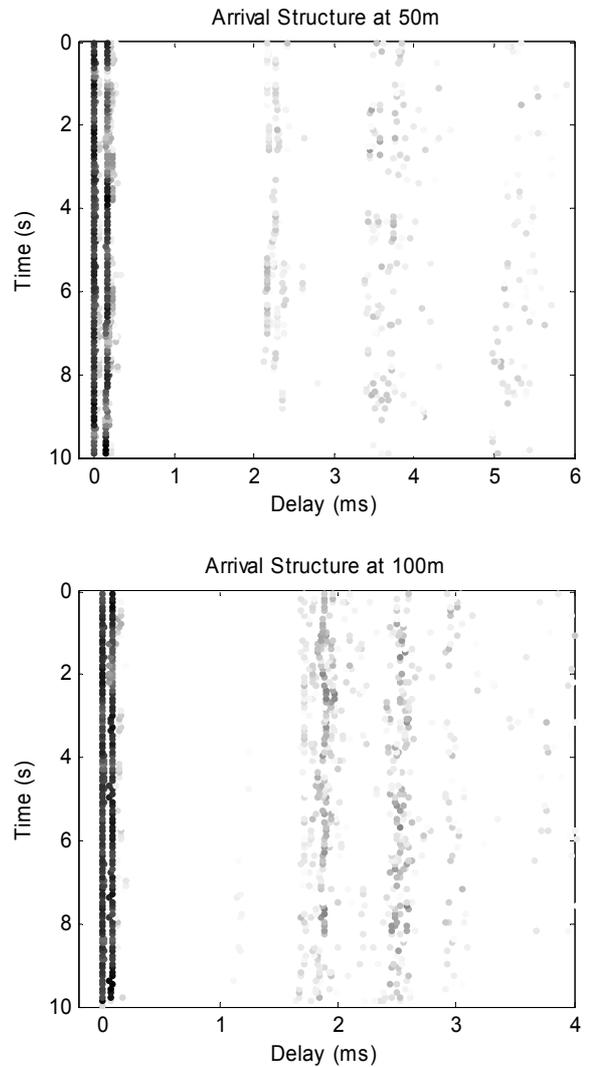
Fig. 6. Multipath arrival structure for 100 signal transmissions at 50 m and 100 m range
