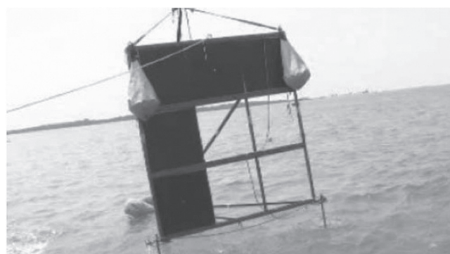
(a) A target frame with 1m x 1m closed-cell Neoprene foam Aluminum-backed reflector panels in an inverted L-shaped arrangement being deployed.
