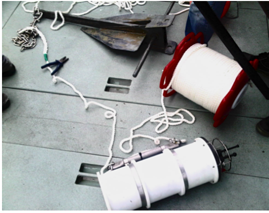
Fig. 8. A UNET-PANDA node being prepared for deployment as a network node in a multihop networking experiment.
