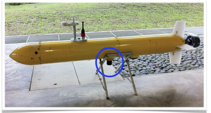
Fig. 5. STARFISH AUV with the UNET-2 modem.
