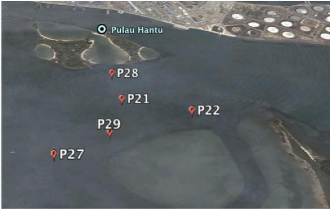
Fig. 3. Five network nodes deployed in Singapore waters. Locations P21, P22, P27, P28 and P29 correspond to the drop locations of the 5 equivalently numbered nodes.
