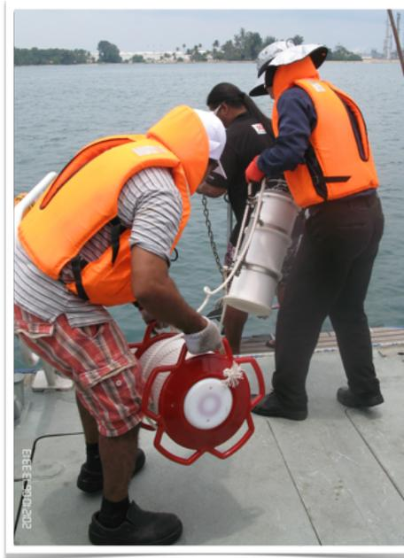
Fig. 1. A Unet-PANDA network node being deployed during the 2012 experiment.
