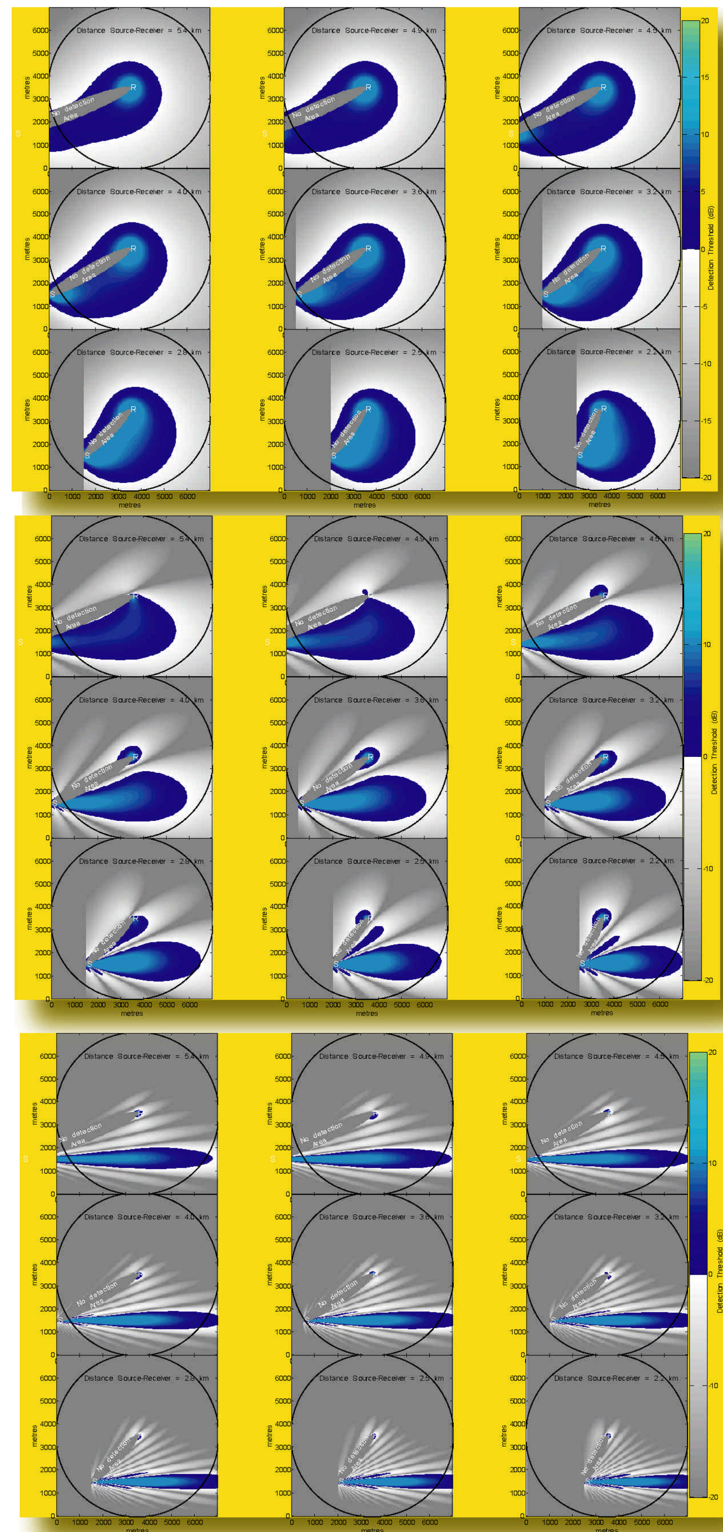
All values relative to 125 dB re 1 \mu Pa-m All 6 figures: Top three: 3D-intensity beam pattern of the piston model used for the Sperm-Whale click production system at the respective frequencies of 1kHz, 3kHz, and 10kHz, from top to bottom. See text for details. Right, from top: Simulation results, where S is the source (a clicking adult Sperm Whale) travelling through the 7km diameter surveillance circle from left to right. The blue area corresponds to the positions where a silent Sperm Whale can be detected by the receiver (R, at the center) thanks to the echo the silent whale produces of the source click. Top figure results are for DI=10dB, middle figure for DI=20dB, and bottom for DI=30dB.
