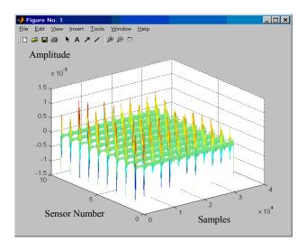
Figure 6. The receivers at the other end receive a multipath reflection of all the pulse trains sent by the source.
