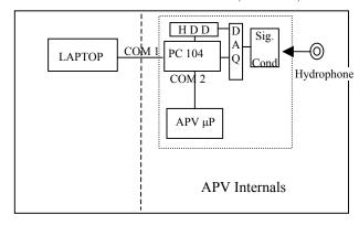
Fig. 9 Block diagram showing interconnections between different electronics blocks
