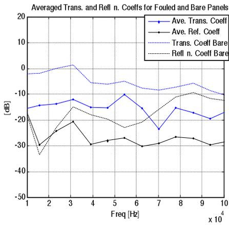
Fig 11: Average Transmission and Reflection Coefficients of Aluminium at 4 weeks
