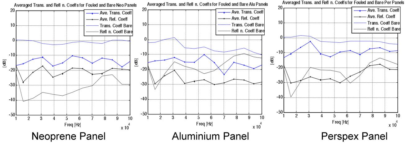
Fig 8: Transmission and Reflection Coefficients of panels after 4 weeks
