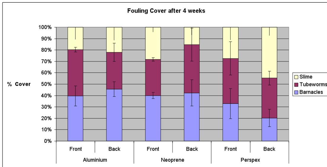
Fig 7: Average Scoring results for Neoprene, Aluminium and Perspex Panels at 4 weeks
