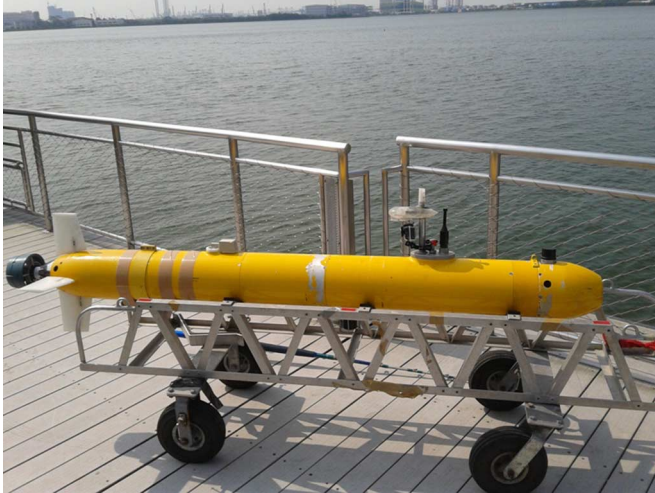
Fig. 4. STARFISH AUV equipped with DVL and LEDIF payload at the Pandan Reservoir, Singapore.
