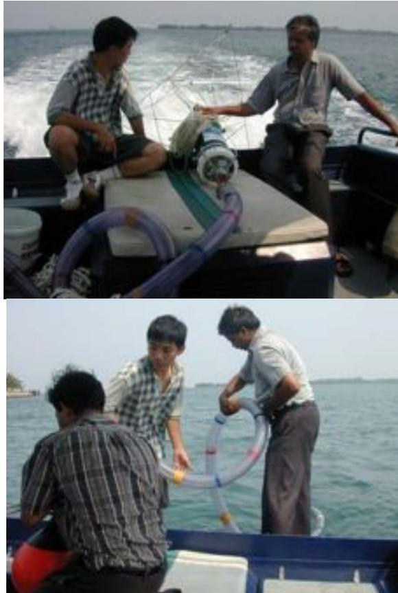
**Figure 39: Deployment of HiDAQ using a tubular spar-buoy**
