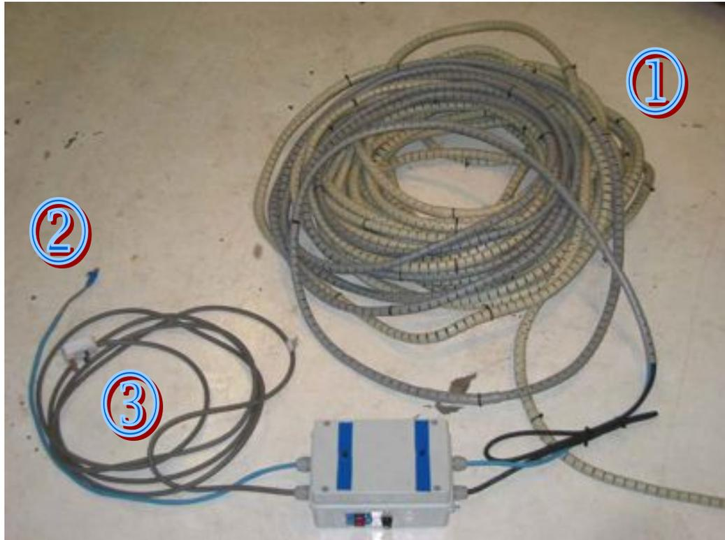
**Figure 7: Fifty meter long underwater cable consisting of a filtered power line and an Ethernet link**
