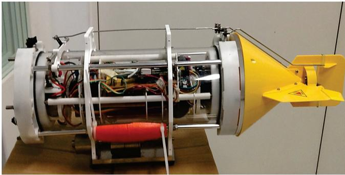
Fig. 20: SwarmBot is the smaller AUV being developed for future team-based operations.
