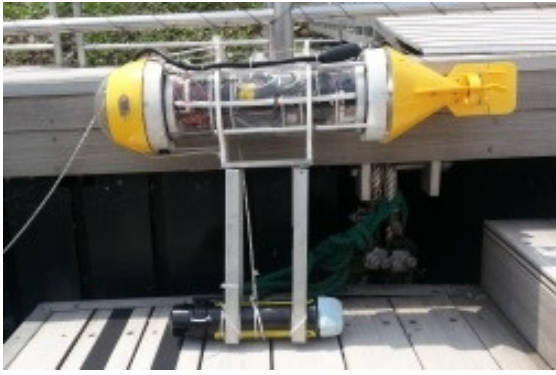
Fig. 9. AUV with transponder strapped to its bottom
