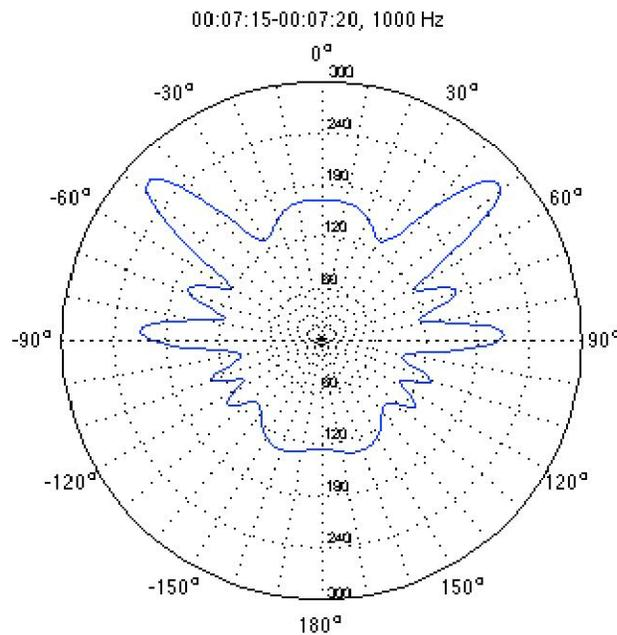
Fig 10 Beamformer output – 1 kHz source
