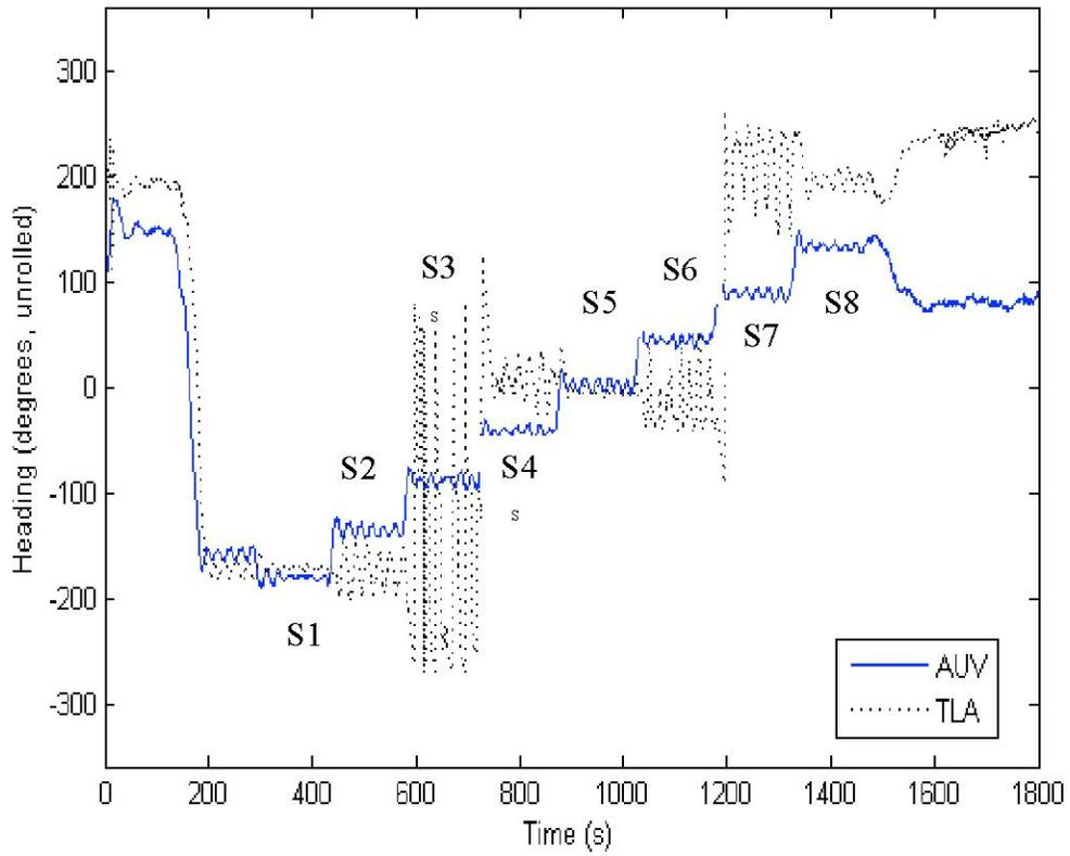
Fig 8 Heading sensor output from the AUV and the array
