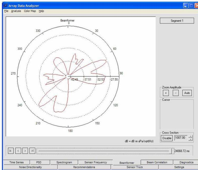
Fig. 3 Beamformer output showing the estimated bearing of two sources separated by  $17^\circ$
