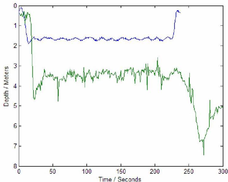
Fig 4 Depth sensor output from the vehicle (blue) and the array
