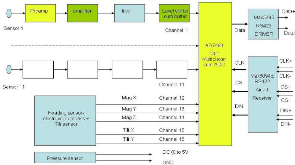
Fig. 2 Block diagram of the array electronics
