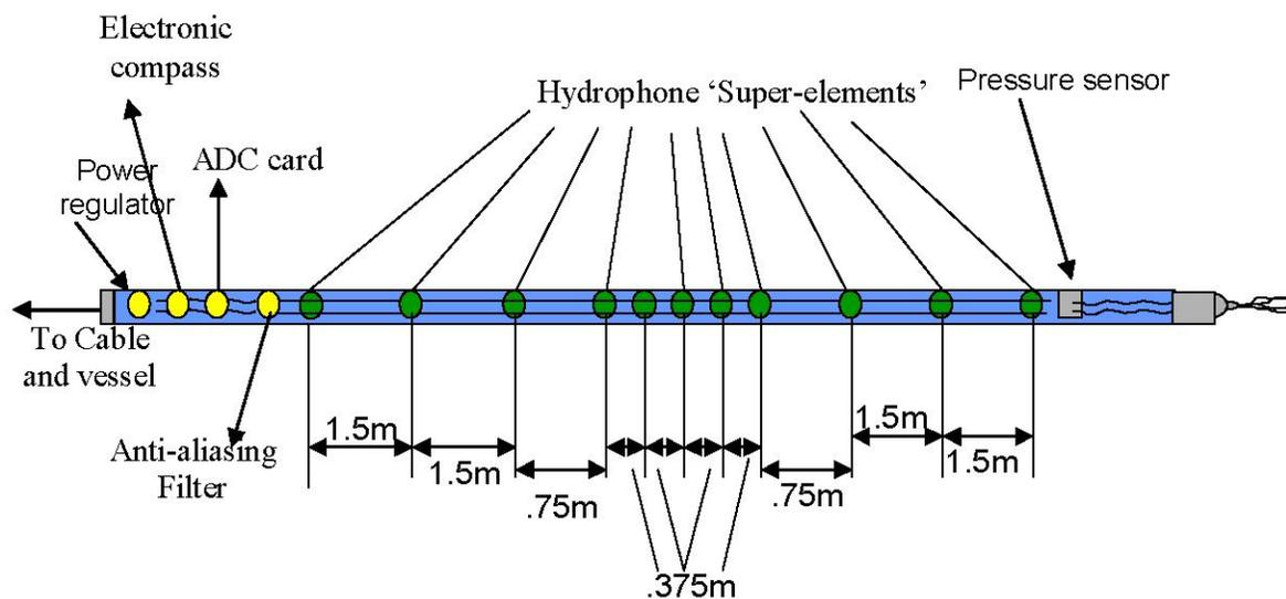
Fig. 1a Schematic of the array showing the layout of various internals
