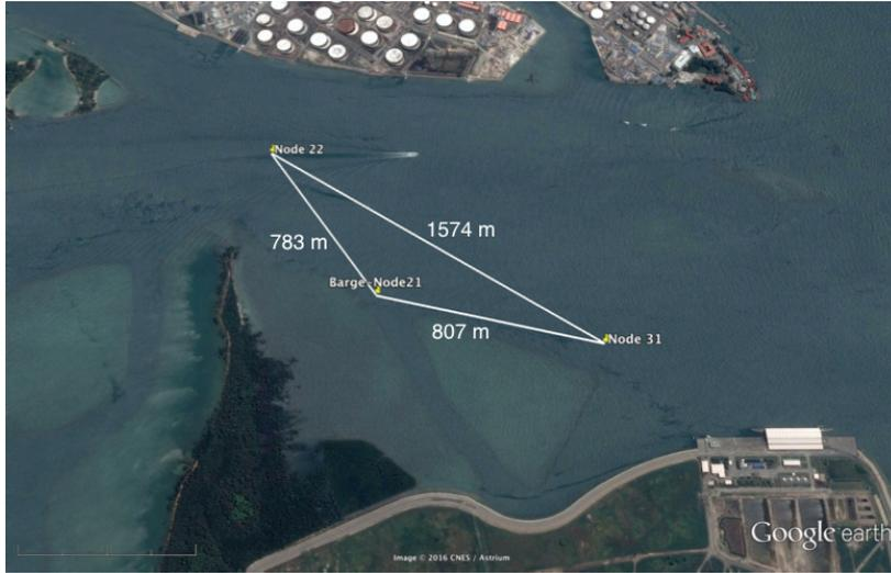
Figure 6.4: UNET network node locations during the experiment in Singapore waters. Yellow markers are network nodes. The links considered for demonstrating Super-TDMA are marked with distances between them.
