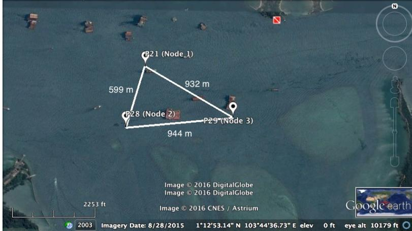
Figure 4.2: UNET network node locations during the MISSION 2013 experiment (deployment #1). White markers are network nodes. The geometry considered for the case study is marked with the distances between the links.
