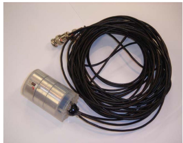
Fig. 4: Photograph of a single crystal hydrophone prototype
