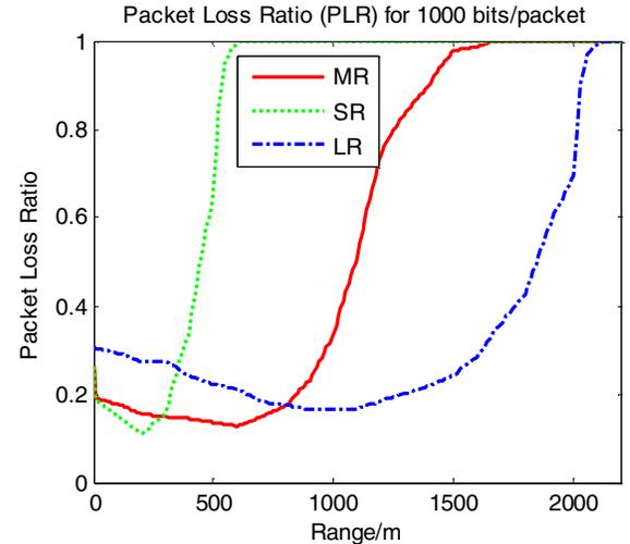
Fig. 3. PLR curves for all channels for 1000 bits per packet. At the optimum range, the packet loss is about 15%.
