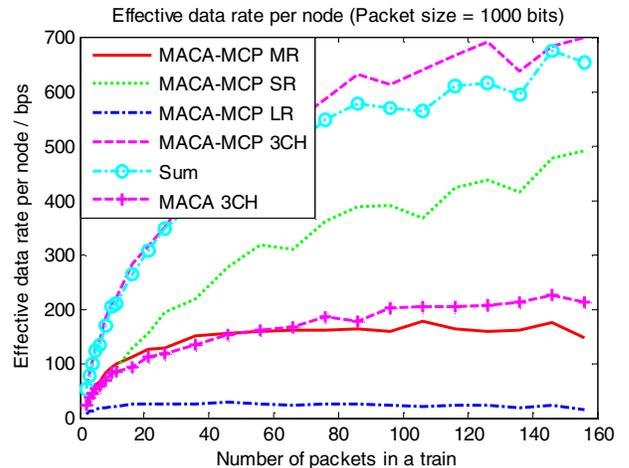
Fig. 7. Effective data rates for the different protocols as a function of packet train size.
