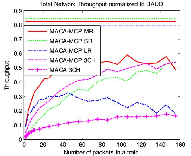
Fig. 8. Network throughput normalized to individual BAUD
