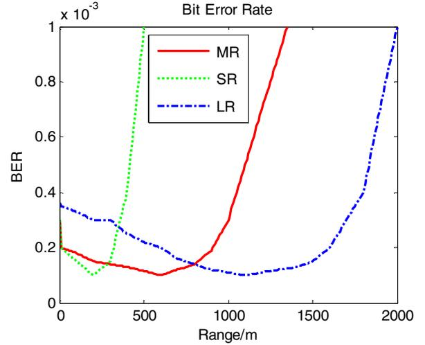
Fig. 1. Coded BER curves for all channels. The BER is modelled as having a rapid increase after their maximum range in this study. At lower ranges the BER increases slightly as compared to each channel's optimum range.
