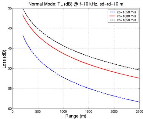
Figure 7. Transmission loss (TL) for various sediment sound speeds representing the minimum (1550 m/s, blue), the mean (1600 m/s, red), and the maximum (1650 m/s, black). At 1 km range, the TL is between 44-53 dB depending upon the sediment speed.
