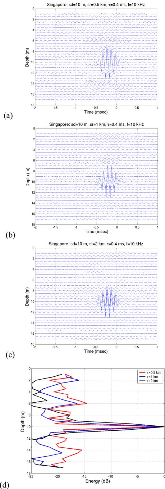
Figure 4. Panels (a)-(c) show signals received on the VRA from time reversed transmission of pulses shown in Figure. 3 (a)-(c), respectively. Plot (d) shows the energy over a 3- ms time window as a function of depth at three different ranges.
