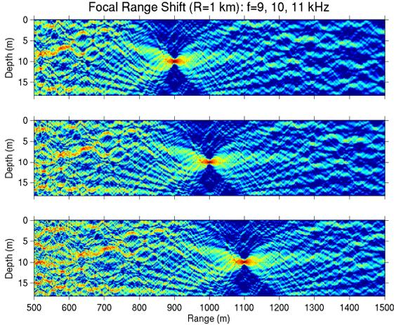
Figure 6. Focal range shift using an appropriate frequency shift. The original PS is at 15 m depth and 1 km range (middle). The top panel shows the focus shifted at 0.9 km range while the bottom panel has a focus at 1.1 km range.
