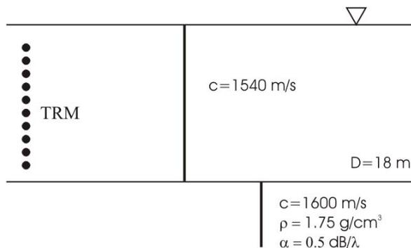
Figure 1. Pekeris waveguide model.
