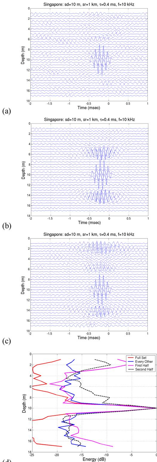
Figure 9. Signals produced from various subsets of TRM transducers when  $N=15$  for a PS at 10 m depth and 1 km range: (a) every other element, (b) first half, and (c) second half. The result using the full set of TRM transducers when  $N=29$  is displayed in Figure. 4(b). (d) displays the energy
