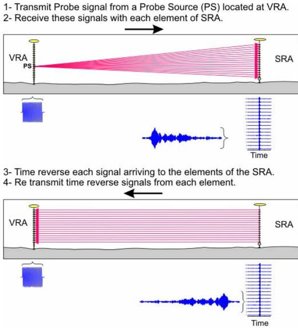
Figure 2. Schematic of a time reversal experiment.
