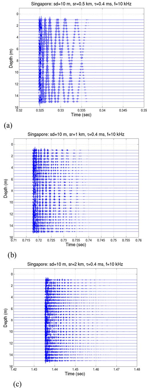
Figure. 3. PS ping captured by the TRM array at three different ranges: (a) 0.5 km, (b) 1 km, and (c) 2 km. Note that the time scales are different.
