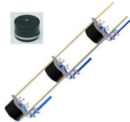
Figure 10 A rendering showing the arrangement of a section of the SRA . On top is the transducer element
