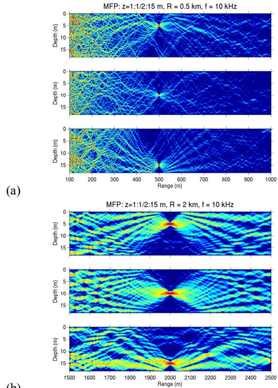
Figure 5. MFP results for three different PS depths (5-m, 10-m, 15-m) at two different ranges: (a) 0.5 km and (b) 2 km.
