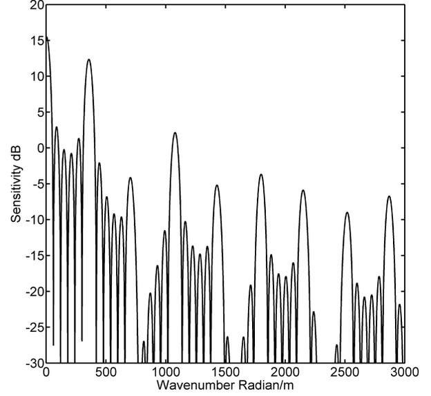
Fig. 2. Wavenumber filtering by DTLA acoustic element
