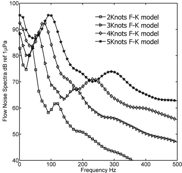
Fig. 4. Estimated level of flow noise at DTLA acoustic element for different tow speeds
