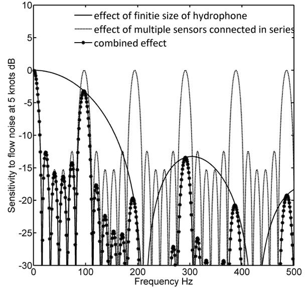
Fig. 3. Flow noise filtering by DTLA acoustic elements at 5 knots
