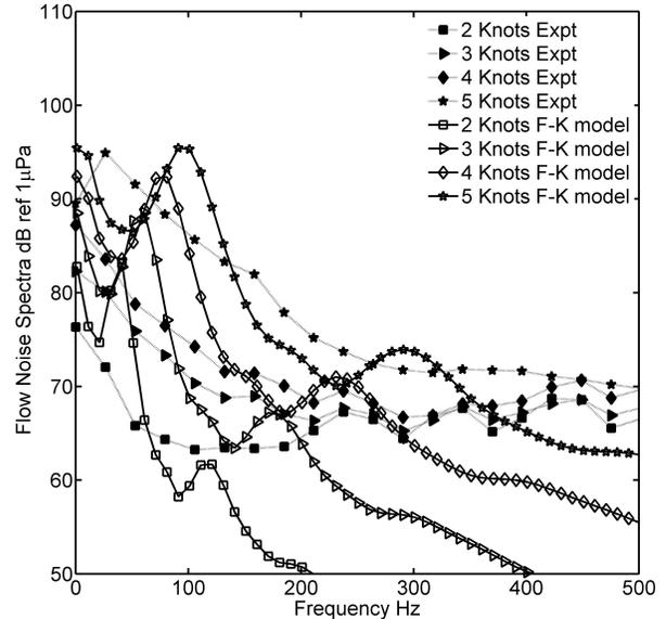
Fig. 5. Comparison of empirical estimate with experimental spectra
