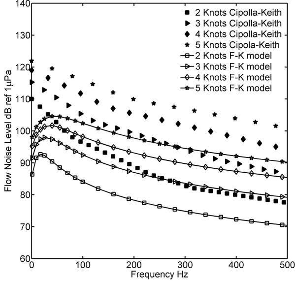
Fig. 1. Frequency spectra of wall pressure fluctuations for DTLA
