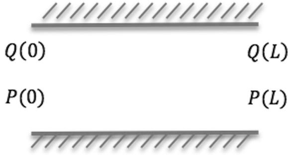
FIG. 3. Linear acoustic 1-D element.
