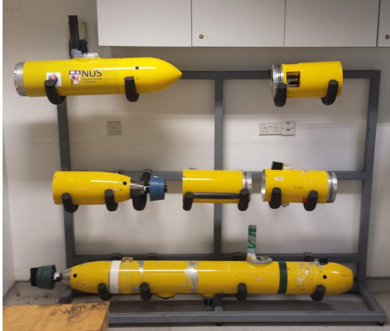
**Figure 1.2:** The STARFISH AUV is highly modular in design which allows easy reconfiguration of vehicle's payloads according to mission requirement.
