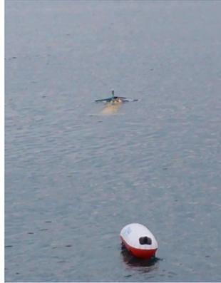
**Figure 5.32:** *STARFISH* AUV was towing a float during the open sea experiment. The picture was taken when the AUV was breaching the surface after completing a dive at 1.5 m depth.
