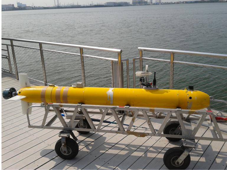
**Figure 1.1:** STARFISH AUV equipped with DVL and LEDIF payload at the Pandan Reservoir.
