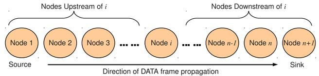
Fig. 3. A  $n$ -hop underwater network with single source and sink, arranged in a linear topology.
