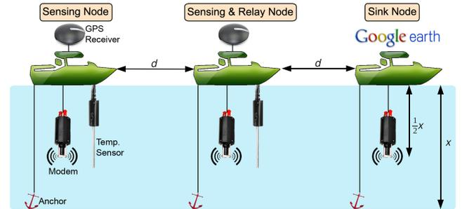
Fig. 9. A 2-hop underwater network with linear topology for a temperature sensing application. The middle node is a pure relay node in our field tests. Inter-nodal distance  $d$  fixed at approximately 150 metres for all tests.
