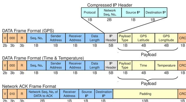
Fig. 2. DATA and ACK frame formats used in our implementation.
