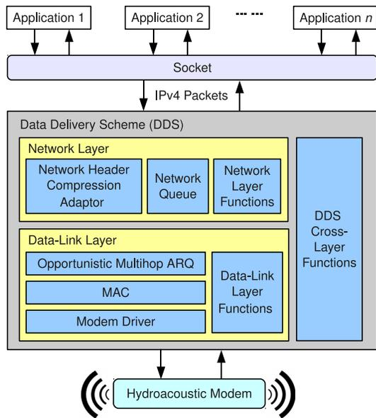
Fig. 1. Software architecture & underwater network stack of the actual implementation.
