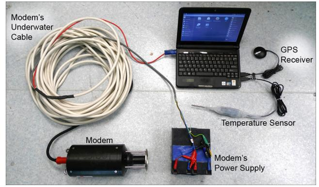
Fig. 8. Experimental setup of a sensing node in the underwater acoustic network. All key components are annotated.
