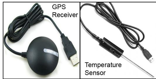
Fig. 5. GlobalSat BU-353 USB GPS Navigation Receiver for obtaining geographical location of sensing nodes. Vernier Go!Temp USB Temperature Sensor for obtaining accurate sea water temperature. Geographical location & temperature information are packed into DATA frames and forwarded along the network to the sink.
