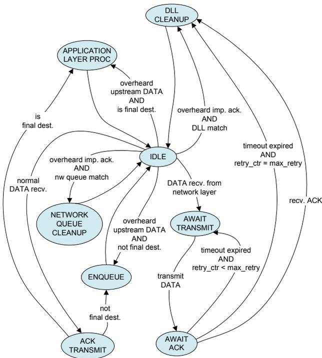
Fig. 4. Protocol state diagram of the opportunistic ARQ with bidirectional overhearing data delivery scheme.
