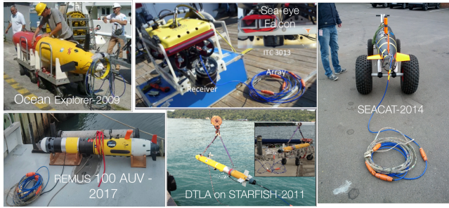
Figure 5. DTLA integrated with different AUV platforms and an ROV platform
