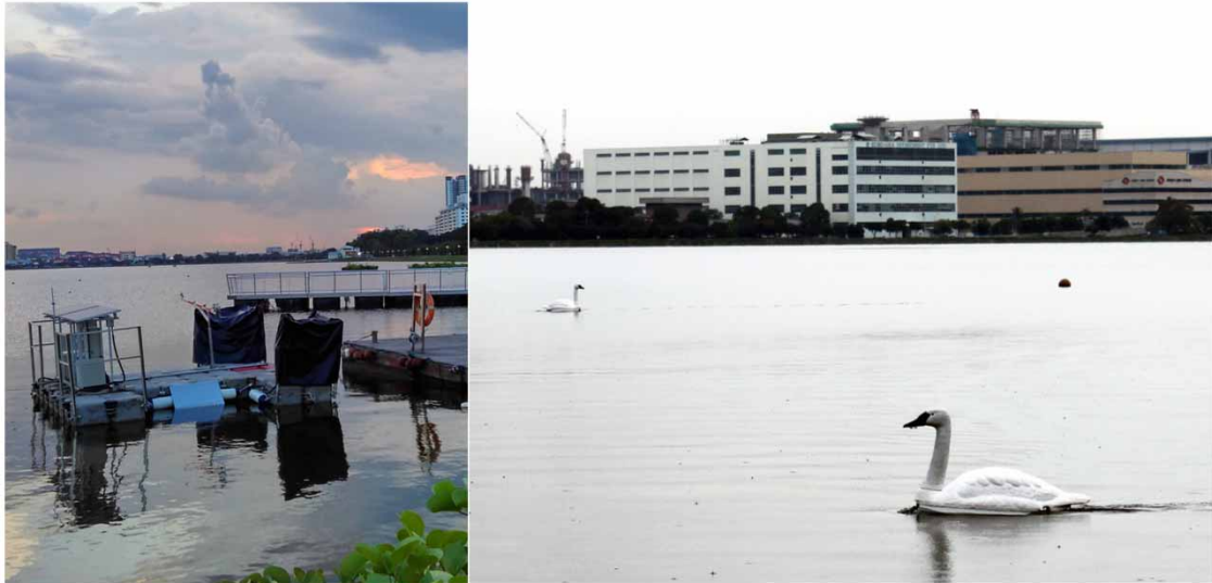
Figure 3 | A customized home-station where NUSwan robots return to, and charge using energy harnessed from solar panels (left). NUSwans executing autonomous missions in a local reservoir in Singapore (right).
