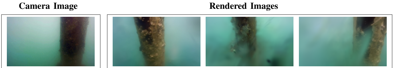
Fig. 13: Camera image and NVS rendered images in the bay near SJI. The rendered images produce photorealistic views of the structure but exhibit some artifacts and noise depending on the camera pose.
