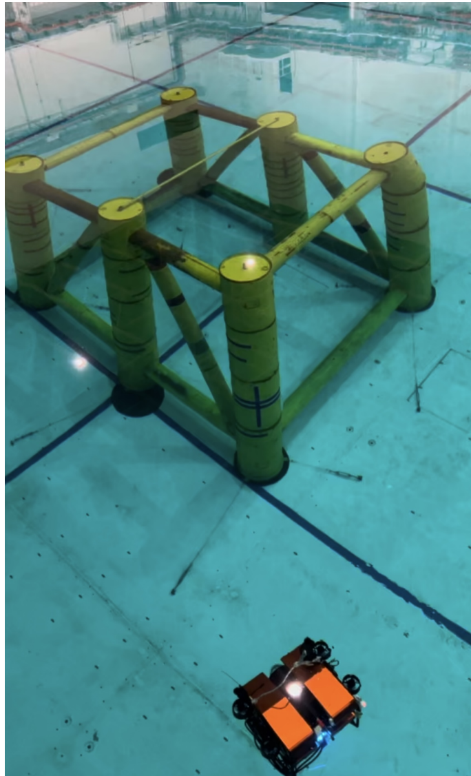
(b) Topview of ROV surveying the structure.
