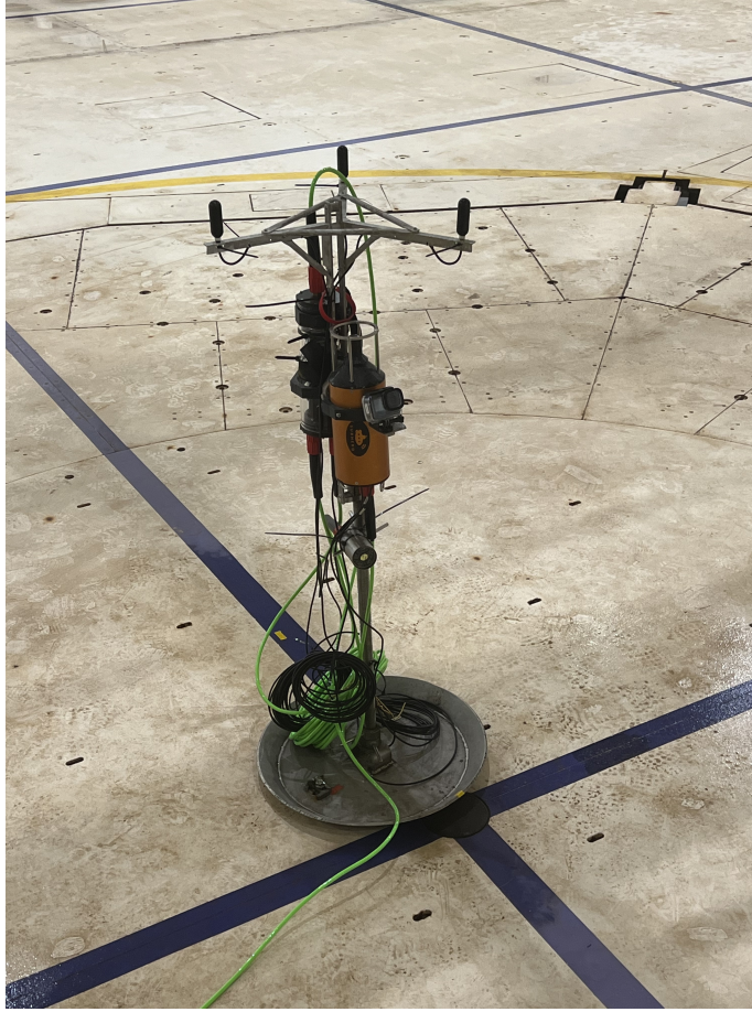
Fig. 5: The USBL setup at TCOMS to estimate the location of the ROV (shown).
