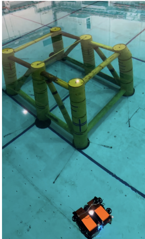
(b) Topview of ROV surveying the structure.
