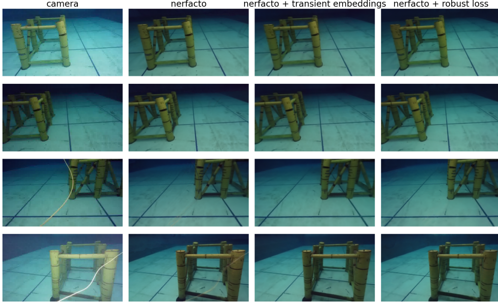
Figure 3.7: Evaluation on the test set of the DOB scene in terms of synthesized novel views from different camera viewpoints, compared to camera ground truth (column 1). The rows indicate the four scenarios, and columns 2-4 show synthesized views from the 3 NeRF approaches. This figure is reproduced from [79].
