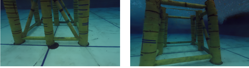
Figure 4.13: NVS rendered images for scenes in TCOMS. The rendered images produce photorealistic views of the structure but exhibit discrepancies in brightness. Some of the rendered views have artifacts in the background as shown in the image on the right.
