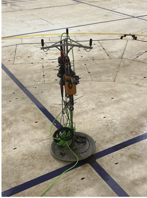
Figure 4.11: The USBL setup at TCOMS to estimate the location of the ROV.
